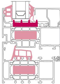
Super High Insulated:  $U_f = 1,53 \text{ W/m}^2\text{K}$
